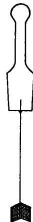
FIG. 1. Stopper with platinum wire and gauze attached as used in the flask combustion method.
